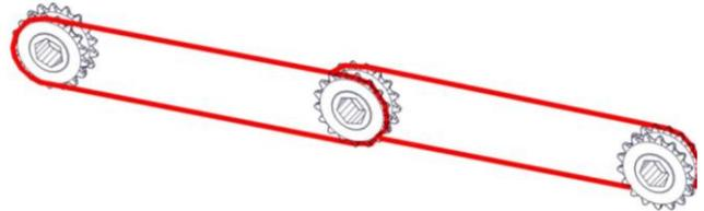
**Step 4:** Add a ½ Inch E-Clip (am-0206) to a Rover Wheel Shaft (am-4133) and slide the shaft through the front bearing and sprocket until the E-Clip is against the bearing.
